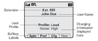
When the handset is in a call or in active mode, information from the telephone system in your facility displays. Information may include extension or telephone number of called or calling party, active line information, and softkeys that have been programmed by your system administrator.
