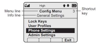
Scroll through menu options by using Nav▲ and Nav▼. When an asterisk (\*) appears to the left of an option, it indicates that the option is currently selected. Press the Exit softkey to return to standby mode. Use the Back softkey to return to the previous menu.
